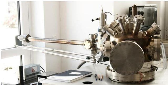
Fig 1: High vacuum chamber
