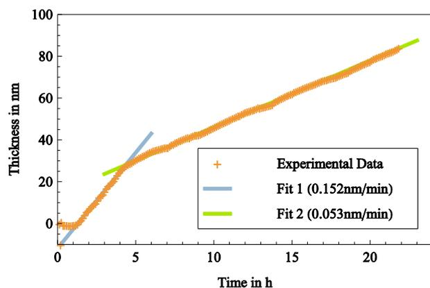
Fig 3: Thickness of the deposited Poly(Bisphenol-A-carbonat) in nm over time in hours
