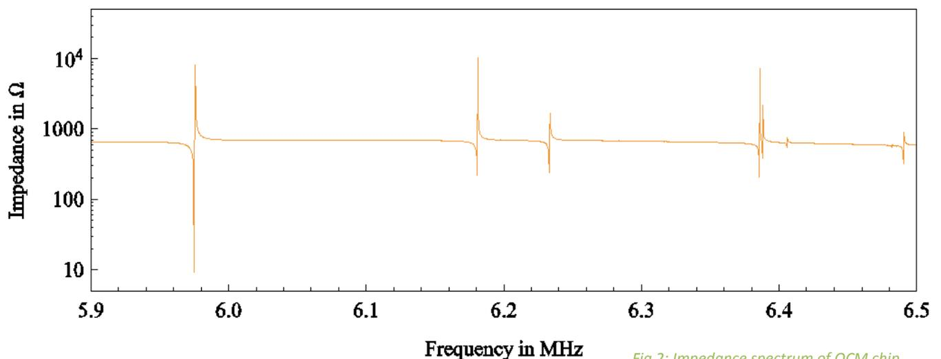
Fig 2: Impedance spectrum of QCM chip
